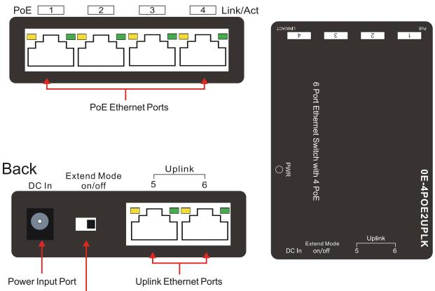
Extend mode ON - supporting long transmssion distance up to 820 ft. (250 meters) with 10mbps for 1-4 ports
